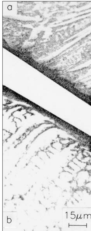
Fig. 3.7 Microstructural features of alloys at the valve/seat insert interface: (a) eatonite insert; (b) alloy No. 6 hardfacing [10]
