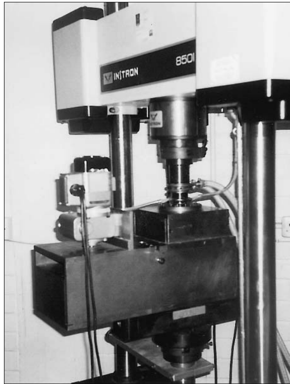
Fig. 5.3 Test rig mounted in a hydraulic test machine
